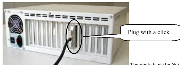
Figure 2.6. Connecting the connection cable to the NOTE-PAC(PCI)F7/F13
